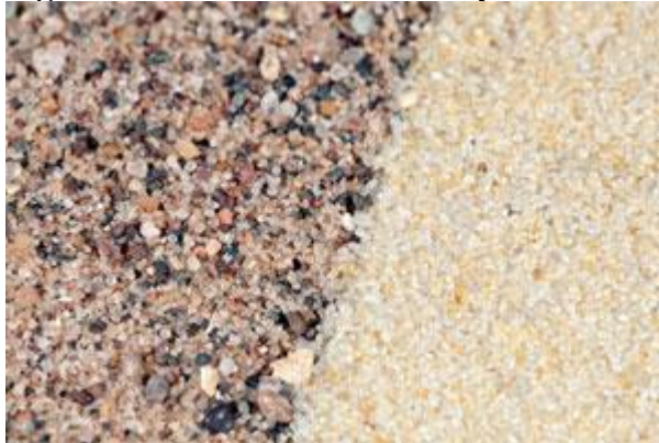
Close-up view of frac sand (on the right) and a typical sand of similar grain size (on the left). Source: iStock
